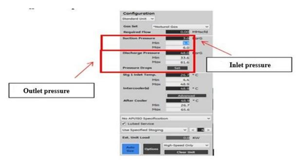
Figure 6: Input of Inlet and Outlet Gas Parameters
